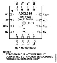
Figure 2. Pin Configuration
