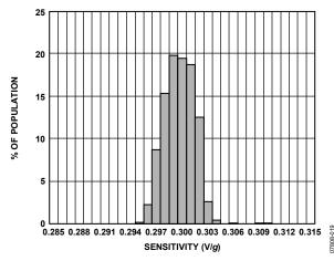
Figure 17. Z-Axis Sensitivity at 25°C,  $V_S = 3 V$
