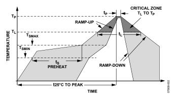
Figure 25. Recommended Soldering Profile
