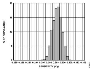
Figure 15. X-Axis Sensitivity at 25°C,  $V_S = 3 V$
