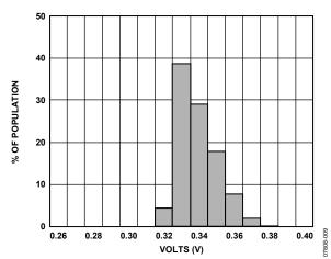
Figure 7. Y-Axis Self-Test Response at  $25^{\circ}$ C,  $V_{S} = 3 V$
